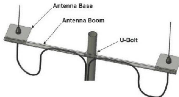
3. Secure cables to top section of mast with tie wraps as shown.
