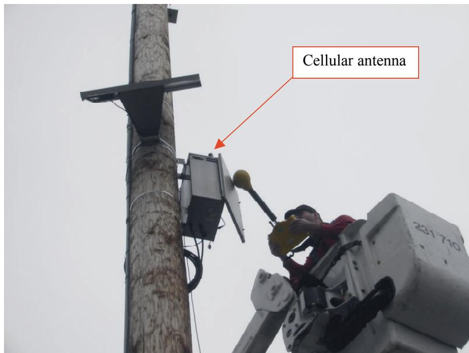
Top: Preparing to measure the 462 MHz DCU power density.
