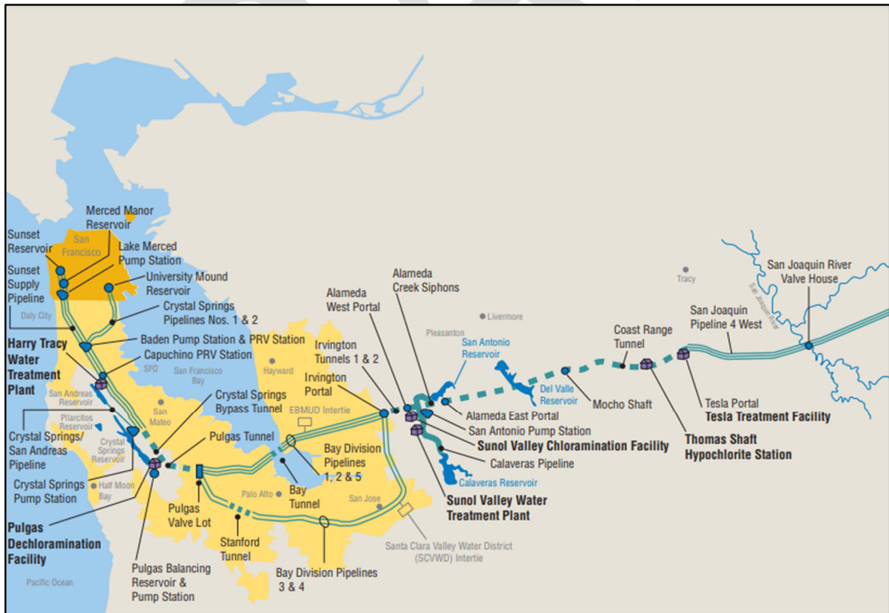
Figure 2-1: Water System Overview
