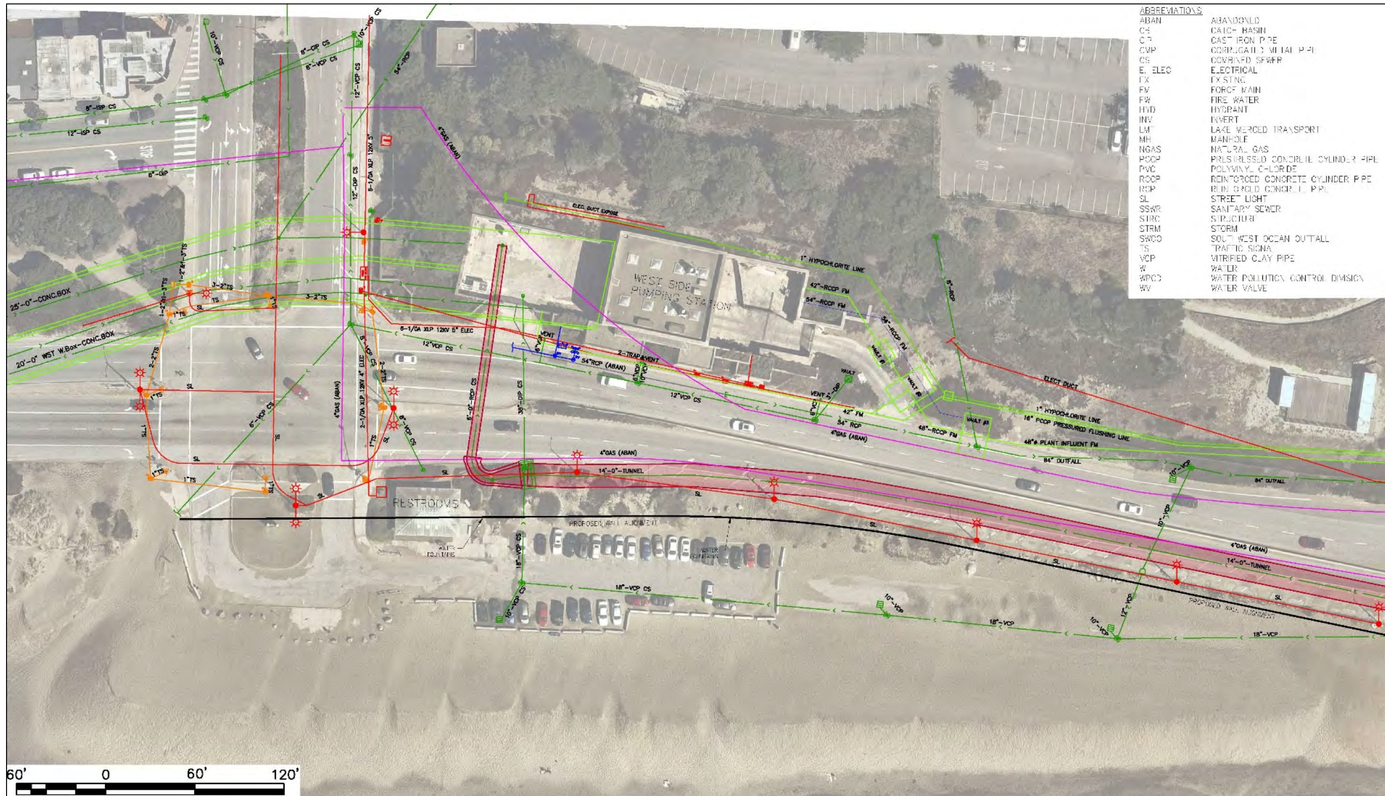
Figure 6-14: Existing Utilities Plan 1.
