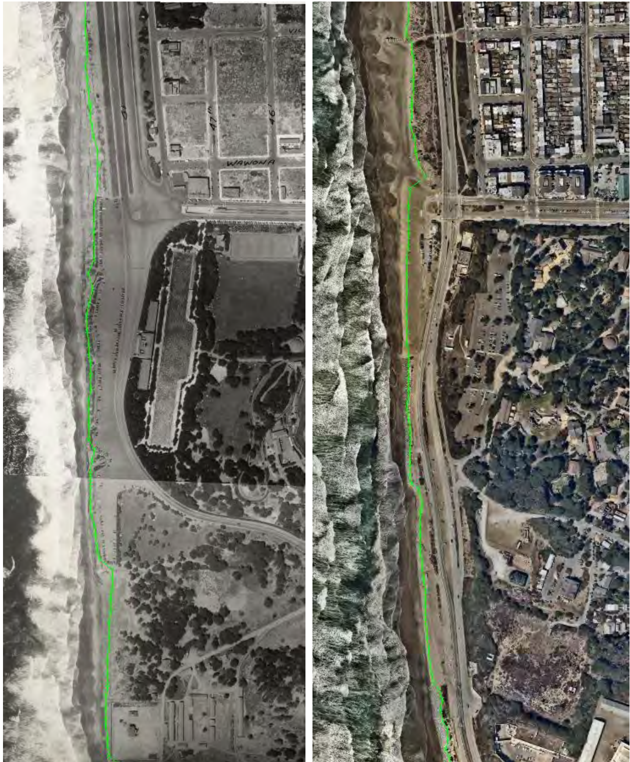
Figure 2-10: Example Delineation of 1938 Bluff Edge (left) and 2019 Bluff Edge (right).
