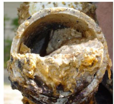
*Sewer pipe clogged from improper grease disposal.*
