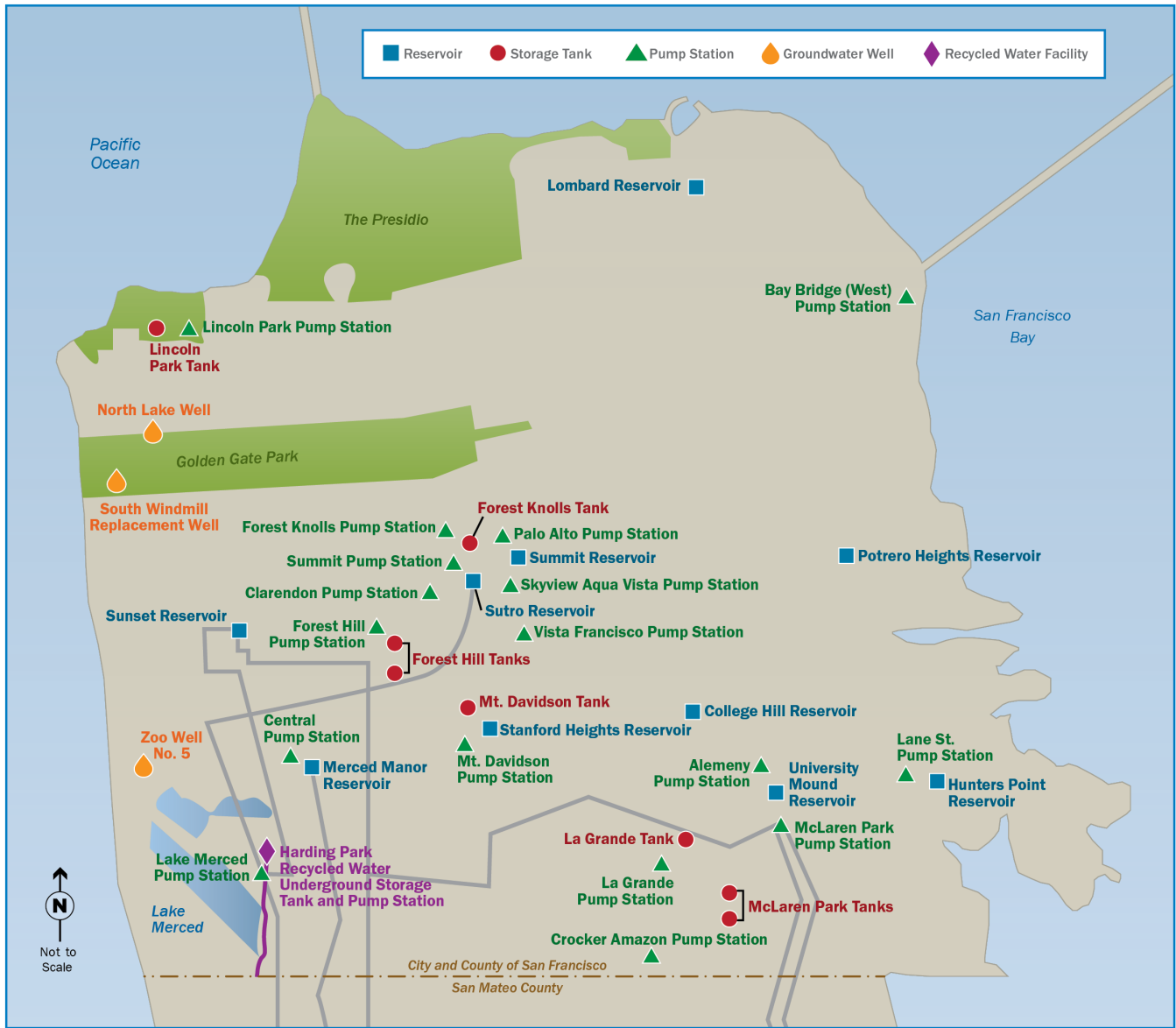
Figure 3-2. In-City Distribution System
