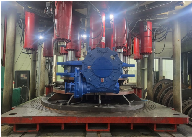
Factory water pressure test of the new 60-inch Butterfly Valve in South Korea
