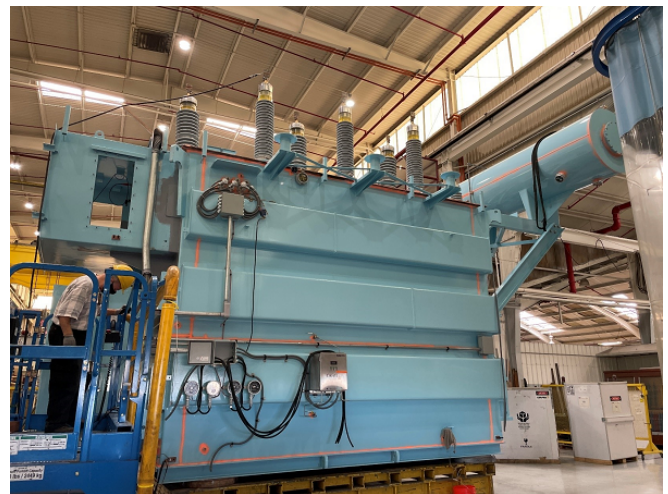
MPH GSU2 (Delta Star F8628) undergoing Final Testing at Factory
