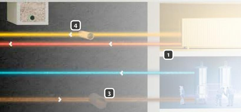
The buildings are connected to the existing water and wastewater main pipes via smaller pipes called laterals. The laterals could remain unchanged but would be connected to the new water and wastewater pipelines. Although not shown on this graphic, the existing underground utilities would be retained and the Civic Center buildings would be able to easily reconnect to the citywide systems if the District systems experienced any problems.
