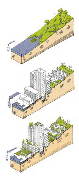
Figure 6. LID seeks to reduce runoff and restore hydrologic function through effective site planning, increased permeability, and landscape-based BMPs.
