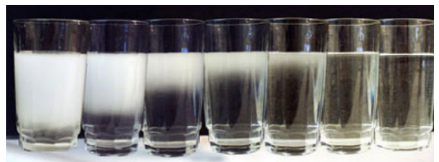
Temporary presence of air in water due to changes in water temperature and pressure (Source: Massachusetts Water Resources Authority, 2020)
