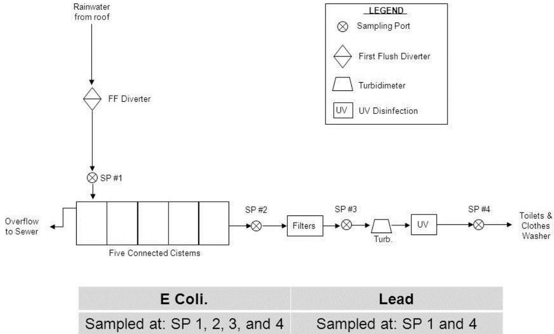
**Figure 1. Kimberg rainwater harvesting system water sampling port diagram.**
