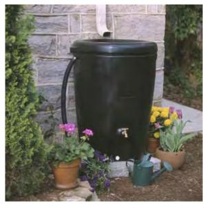
A disconnected downspout and rain barrel. Photo: Clean Air Gardening
